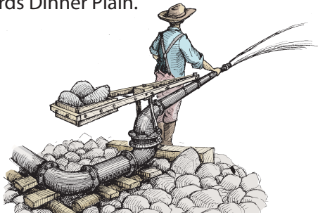
Hydraulic sluicing using pressurised water from the ditch (A Swift)
